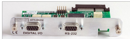
KTTI-RS232 RS-232 interface with 6 digital I/O ports.
